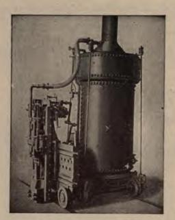
The Ingersoll-Sergeant Improved Stone Channeling Machine. Used in Stone Quarries for producing dimension
